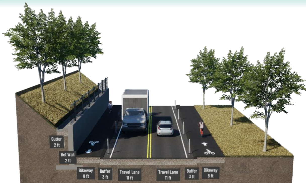
Figure 12: Cross Section for At-Grade Class IV Bikeway with Cut Section
