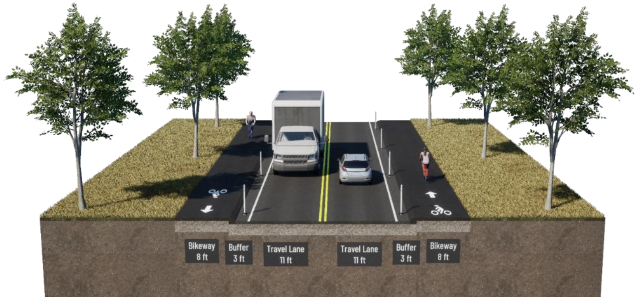
Figure 11: Cross Section of At-Grade Class IV Bikeway
