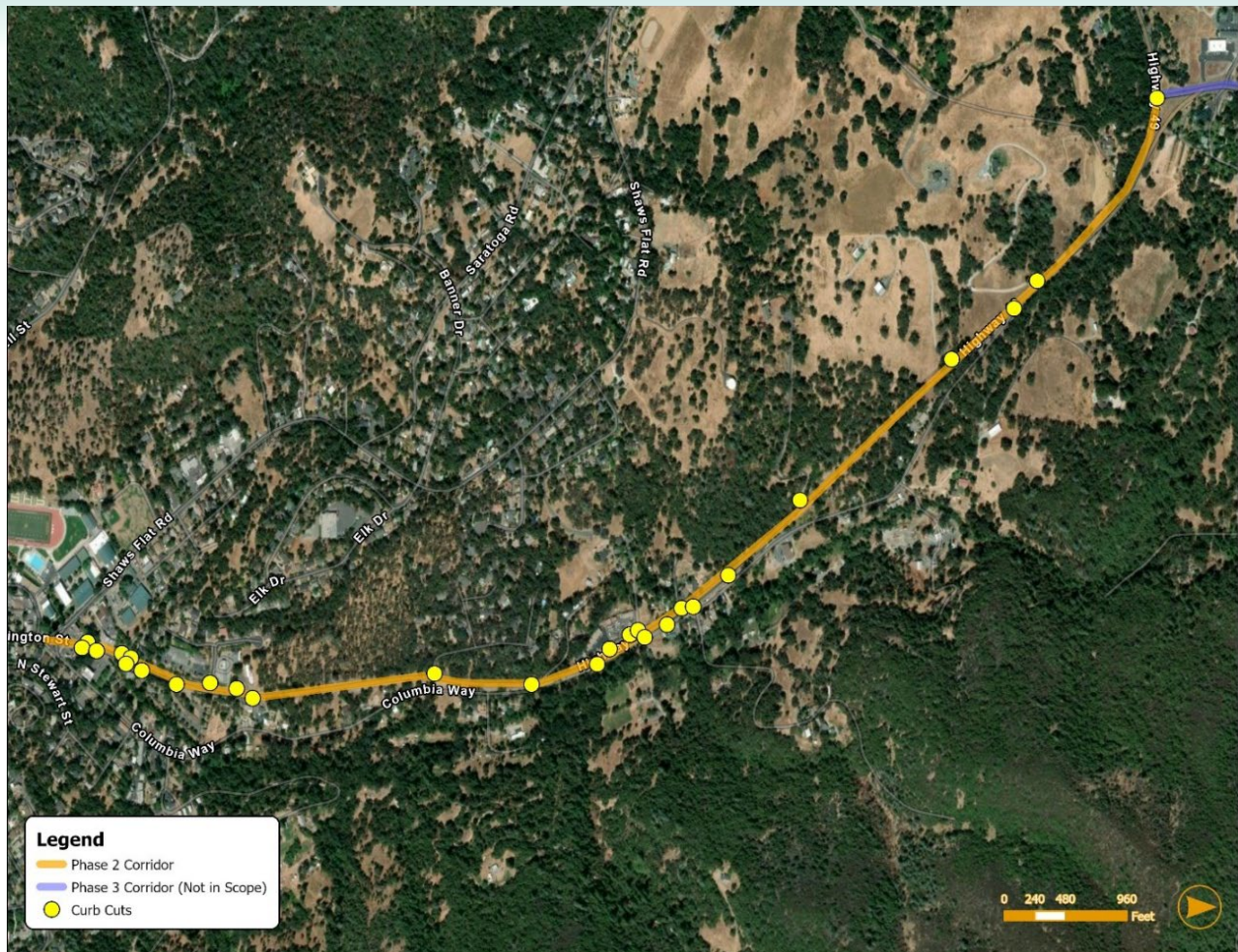
Figure 21. Curb Cuts Bisecting SR 49 (Kimley-Horn, 2025)
